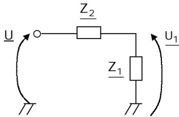
$$\underline{U}_1 = \frac{\underline{Z}_1}{\underline{Z}_1 + \underline{Z}_2} \underline{U}$$
